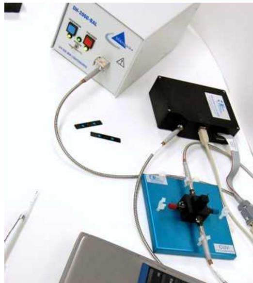
Figure 3 Ocean Optics HG4000 Spectrometer
