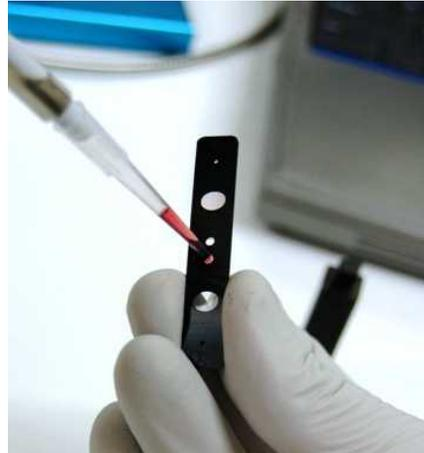
Figure 2: Filling the SpecVette
