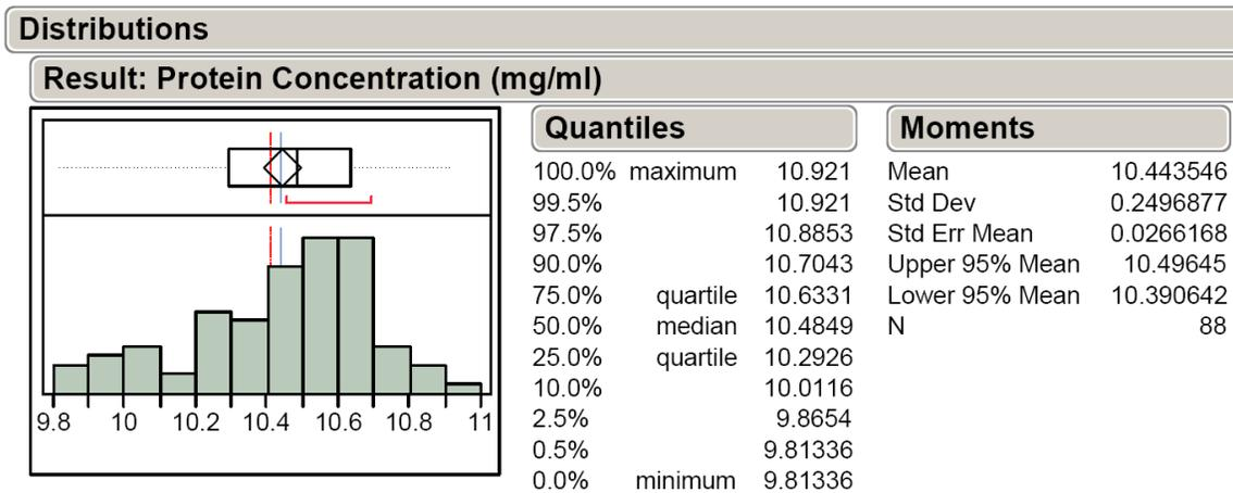
Figure X: Histogram of SpecVette Data with 1 mm Pathlength Quartz Grand Mean (10.41 mg/ml, Red Line) and SpecVette Grand Mean (10.44 mg/ml, Blue Line) Indicated.
