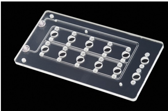
Figure 4. Top view of the cell culture card that flew on NASA's GeneSat experimental satellite to demonstrate autonomous cell culture in near earth orbit. The fluidic card is constructed from layers of acrylic bonded with an optically clear bottom and a gas permeable top. A single inlet distributes nutrients evenly across all ten sample chambers. The system flew in December 2006 and successfully telemetered data on cell growth to earth.
